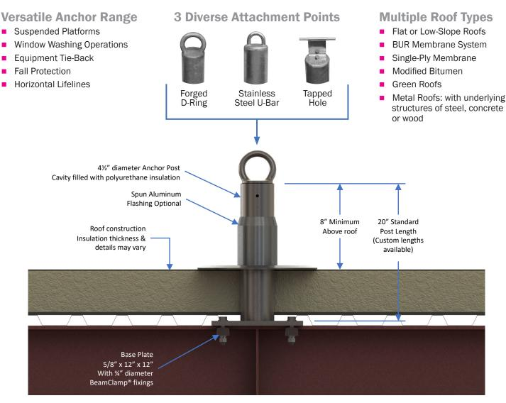
Use Kee Safety flashings with Kee Safety anchors for best compatibility.
