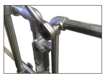
I. Carefully re-position the gate top and bottom tubes into the cast fittings. Use a spirit level, to ensure the gate is level. Tighten the cast fittings grub screws using a hex head socket. Using the torque wrench ensure the castings are torqued to 39Nm.
