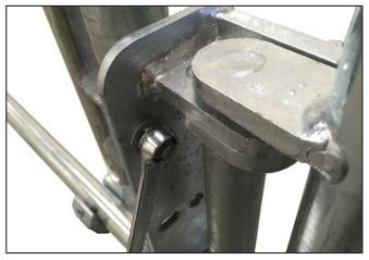
**B.** Using a 11/16" or ½" flat washer and nut connect the U bolt to the Support Leg/Structure and tighten.
