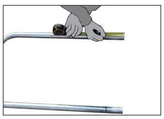
**G.** Divide the distance recorded in step **E** by 2, mark this measurement on gate top and bottom tubes as shown. This measurement is to be removed from both gates to ensure both gates are the same width and meet in the middle.
