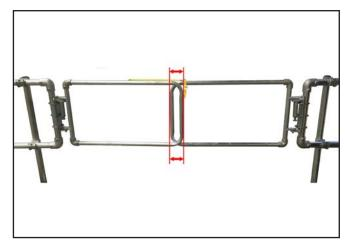
**E.** To cut the gate to the correct size simply place a straight edge/magnetic level as shown and measure the distance between the outside edges of the vertical tube on both gates. **(DO NOT CUT AT THIS MARK!)**
