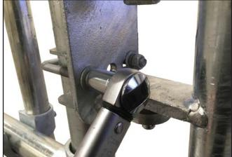
**D.** Torque all nuts/U Bolts to 39Nm using the 11/16" or  $\frac{1}{2}$ " socket and torque wrench.
