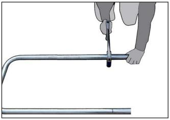
H. Using a hacksaw or similar carefully cut through the top and bottom tubes as shown. For galvanized assemblies, spray with Galvafoid or similar to prevent corrosion.
