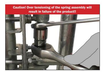
**L.** Using the 15/16" socket & ring spanner start to tighten the bolt until the gate completely closes. (Note:-You may have to hold the socket whilst using the ratchet). Once the gate is completely closed tighten the locking nut to hold the tension. Caution:- Continue to hold the ratchet firmly and do not release until the lock nut is tightened. Now remove the socket and spanner from the hinge. Repeat as necessary, to ensure that the gate closes sufficiently, once opened and released.
