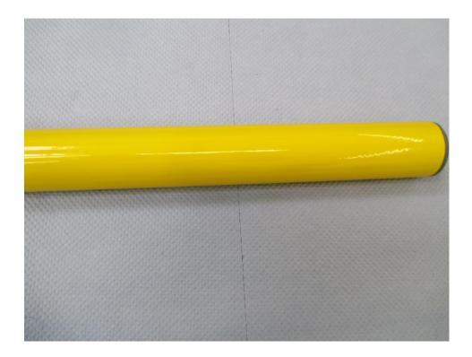
Fig 3: Photograph showing the condition of the 33.7 x 250mm Tube Sample after 216 hours Salt Spray Test
