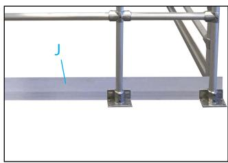
$\textbf{10.} \ \, \text{Add part (J) toe-board onto both left and right hand side frames using M10 x 50mm bolts and nuts provided.}$
