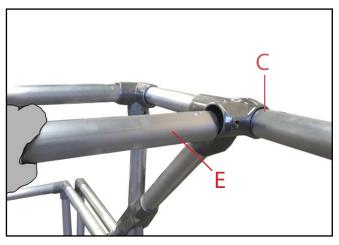
**8.** Insert 2no. part (**E**) horizontal tube to link up left and right hand cantilever sections. Tighten grub screws using hex key.
