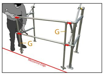
**8.** Slide part ( $\mathbf{G}$ ) vertical uprights to the left and right hand side of horizontals as shown above. Tighten using 1/4" hex key.
