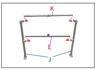
**2.** Build 2 frames using 2no. (**J**) uprights, 1no. (**E**) horizontal for the lower horizontal and 1no. (**K**) for the upper horizontal per frame. Once tube is fully inserted tighten grub screws using 5/16" hex key.
