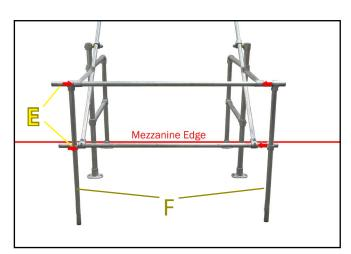
**9.** On opposite end to mezzanine edge slide 2no. part (**E**) horizontal through cantilever tube ends. Add 2no. (**F**) uprights onto ends of horizontal tubes. Tighten using 1/4" hex key.
