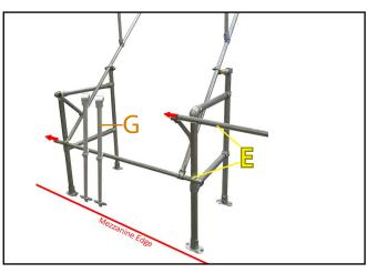
**7.** On Mezzanine leading edge slide 2no. part (**E**) horzontal tubes through the cantilever tube ends. During this process add 2no. part (**G**) vertical uprights with toe-board brackets onto horizontal tubes part (**E**).
