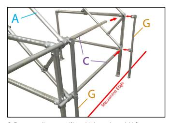
**6.** Rotate cantilever part (**A**) so this is as above. Add 2no. part (**C**) horizontal tubes on mezzanine edge end and add part (**G**) upright tubes as above onto parts (**C**) during the process.
