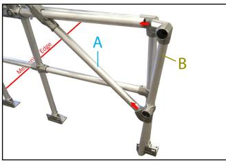
**7.** Add part **(B)** upright tubes onto opposite end of part **(A)**, insert tubes into fittings as per above and tighten grub screws using hex key.
