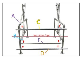
**11.** On opposite end to mezzanine edge mount horizontal tube part ( $\mathbf{C}$ ) to upper cantilever rails ( $\mathbf{A}$ ). Slide part ( $\mathbf{F}$ ) 5.9" up part ( $\mathbf{B}$ ) cantilever tubes and tighten using 1/4" hex key. Mount horizontal tube part ( $\mathbf{D}$ ) to lower cantilever rails ( $\mathbf{B}$ ). Tighten fittings using 1/4" hex key.
