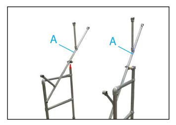
**5.** Take part (**A**) with bearing attached and with gate rail on inner side mount to the vertical tube of the frame. Ensure bearing is facing mezzanine edge side as per diagram above. Repeat this step for other frame.
