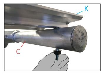
**11.** Add 1no. part ( $\mathbf{K}$ ) toe-board to part ( $\mathbf{C}$ ) uprights. Thread M10 x 80mm bolt through hole in upright and add nut and washer. Tighten to 15Nm.
