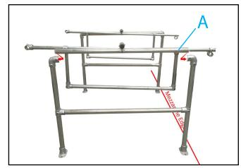
**5.** Take part (**A**) with hinge arm and mount wide size 8 (1.90" dia) tube to frame with gate rail on inner side. Repeat this step for other frame. NB. Slight loosening of the frame may be required to allow the horizontal to be inserted into the frame.
