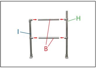
**2.** Build 2No frames using 1No. (**H**) upright, 1No. (**I**) upright and 2No. (**B**) horizontal parts per frame. Once tubes are fully inserted tighten grub screws using 5/16" hex key.
