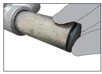
**11.** Place plastic end caps on all exposed tube ends. These may need to be tapped into place using a rubber mallet.
