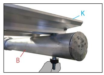
**12.** Add 1no. part ( $\mathbf{K}$ ) toe-board to part ( $\mathbf{B}$ ) uprights. Thread M10 x 80mm bolt through hole in upright and add nut and washer. Tighten to 15Nm.
