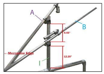
**6.** Carefully measure and mark 12.20" from top of frame as shown above. Slide part (**B**) onto part (**I**) and mount fitting at this mark, ensuring bearing is on the inside of the frame then tighten grub screw. Measure and mark 9.45" from top of fitting on part (**B**). Add part (**A**) to part (**I**) mouting the fitting to this mark ensuring bearing is facing same direction and tighten grub screw. Repeat process for other frame.
