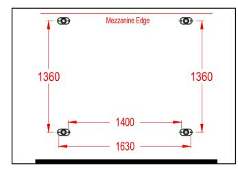
**1.** Using the above guide mark the position of the holes. Carefully drill a 12mm hole on each mark. Remove any debris using suitable extraction equipment.
