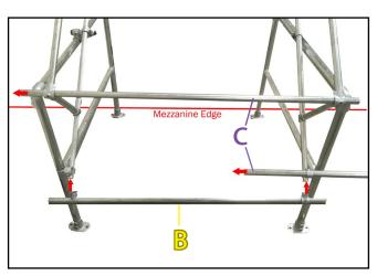
**7.** On opposite end to mezzanine edge add 2no. part ( $\mathbf{C}$ ) horizontal tubes to upper and lower cantilever tubes. Then add part ( $\mathbf{B}$ ) onto ends of lower cantilever tubes. Tighten using 1/4" hex key.
