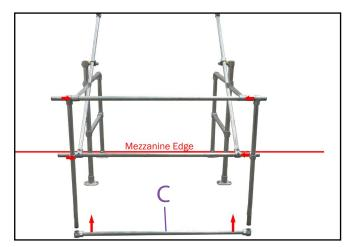
**12.** On opposite end to mezzanine edge insert part ( $\mathbf{C}$ ) horizontal tube by sliding tube 4" up the vertical posts. Tighten using 1/4" hex key.
