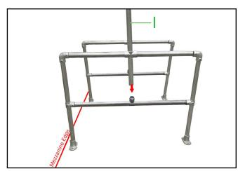
**5.** Slide part (I) upright rail through fittings on each frame. Tighten grub screws. Repeat for other frame.
