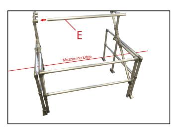
**9.** Repeat process for other side of gate using 3no. part (**E**) horizontal tubes. Once tubes have been inserted tighten grub screws and torque to 39Nm.
