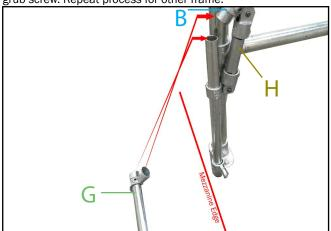
**9.** Add part (**H**) upright by sliding fitting onto end of part (**B**) on mezzanine leading edge end of the gate and tighten grub screw. Then linking part (**G**) horizontal tube to exposed tube ends on part (**H**) and part (**B**). Tighten fittings using 1/4" hex key.
