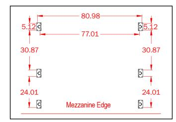
**1.** Lay components on safe flat working area. Using adiquate fall protection device drill 12mm holes to allow feet to be attached using the above guide.
