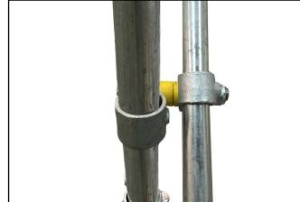
**7.** Ensure frame is parallel. If not, the gate will not operate smoothly. Adjust as necessary by rotating the fittings.
