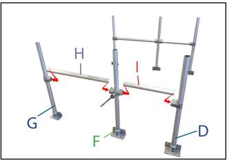
**2.** Build 2 frames using 1no. (**D**) part, 1no. (**F**), 1no. (**G**) per frame as above. Link upright posts using 1no. part (**H**) and 1 no. part (**I**) per frame and tighten grub screws using 5/16" hex key. Repeat process to make second frame.
