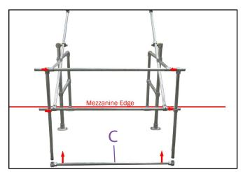
**12.** On opposite end to mezzanine edge insert part ( $\mathbf{C}$ ) horizontal tube by sliding tube 100mm up the vertical posts. Tighten using 1/4" hex key.
