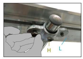
**12.** Mount toe-board (**L**) to part (**H**) uprights by sliding 4no. bolt heads along back of toe-board and then inserting 2no. bolts into each fitting. Loosely add washer and nut allowing movement within the toe-board for adjustment in next step.
