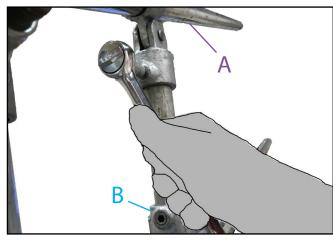
**8.** Connect cantilever tube link post form part (**B**) and connect into fitting on part (**A**). This will link the two tubes and allow the concertina action.
