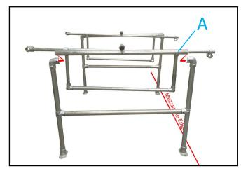
**5.** Take part (**A**) with hinge arm and mount wide size 8 (48.3mm dia) tube to frame with gate rail on inner side. Repeat this step for other frame. NB. Slight loosening of the frame may be required to allow the horizontal to be inserted into the frame.
