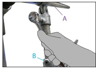
**8.** Connect cantilever tube link post form part (**B**) and connect into fitting on part (**A**). This will link the two tubes and allow the concertina action.
