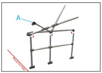
**5.** Add part (**A**) cantilever arms onto the frame, ensuring that the arm is positioned on the inside of pallet gate. Repeat for opposite frame.
