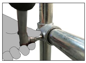
**13.** Ensure to fittings are torqued to 39Nm, that the pallet gate operates smoothly and is balanced.
