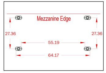
**1.** Using the above guide mark the position of the holes. Carefully drill a 0.5" hole on each mark. Remove any debris using suitable extraction equipment.
