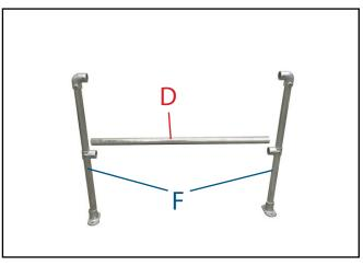
**2.** Build 2No frames using 2No. (**F**) uprights, 1No. (**D**) horizontal per frame. Once tubes are fully inserted tighten grub screws using 5/16" hex key.
