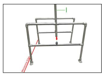
**5.** Slide part (I) upright rail through fittings on each frame. Tighten grub screws. Repeat for other frame.
